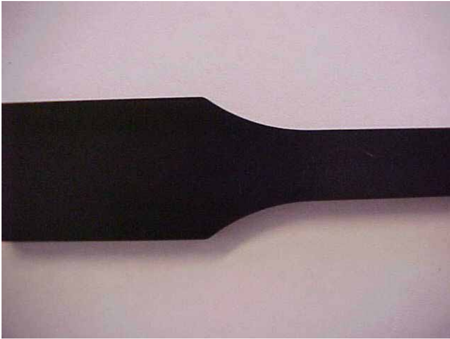
Figure 2. Tensile dumb-bell specimen injection moulded using AX 06 009 material (Creasolv trial after 4 th pass through ring extruder)
