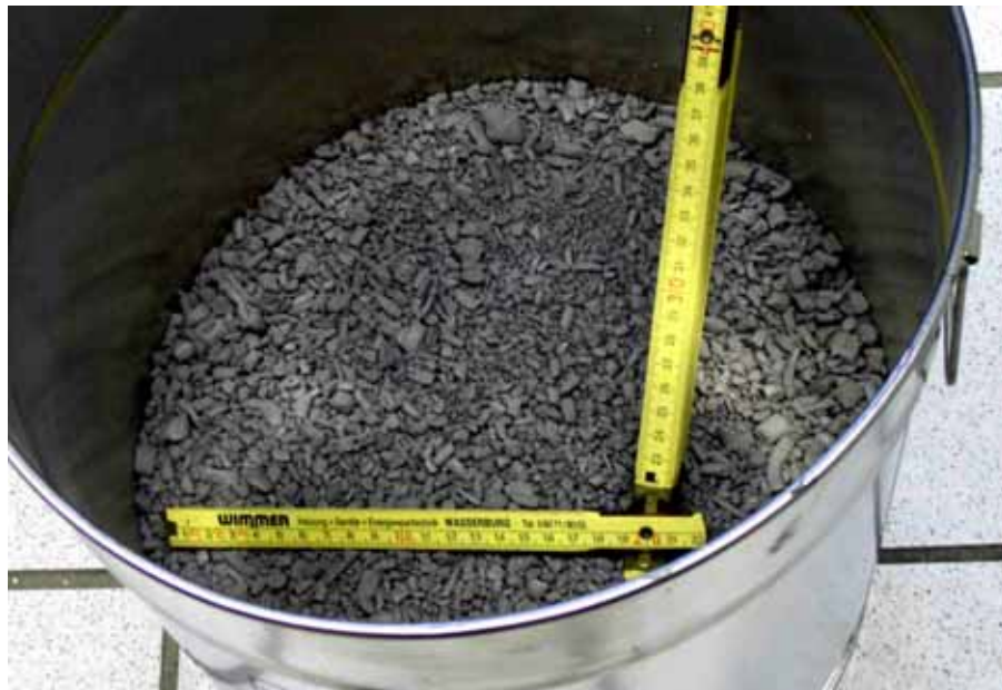
Creasolv TV casing Trial 1 – precipitated debrominated polymer
